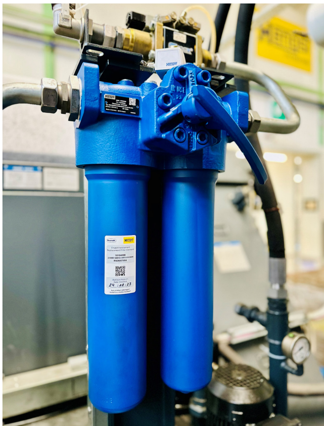
Filter elements are easy to recognize: Practical sticker directly on the filter housing Picture source: Hengst Filtration
