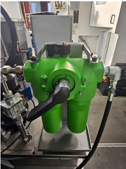
Duplex filter Pi 370 from Filtration Group Industrial Picture source: Belki Filtertechnik GmbH
