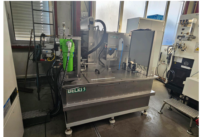
View of the BFA filter system with FG duplex filter Pi 370 Picture source: Belki Filtertechnik GmbH
