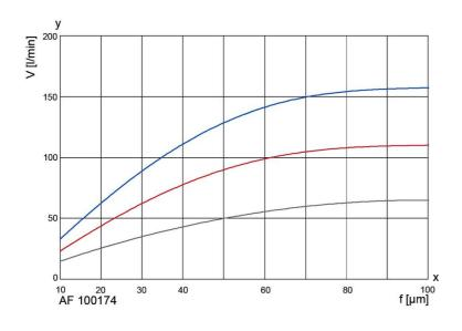
The curves indicate the volume flow ferred to a differential pressure of 0.3 bar. to guarantee reliable operation of an auto-
