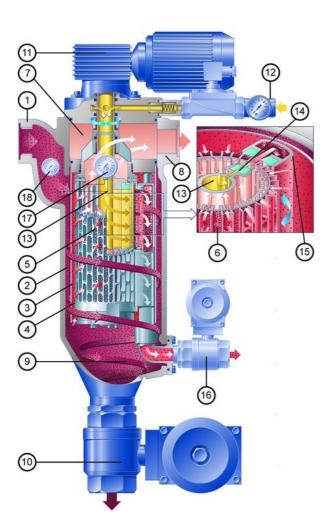
The filter is cleaned when a preset differential pressure limit, a set interval or a defined filtered fluid quantity is reached.
