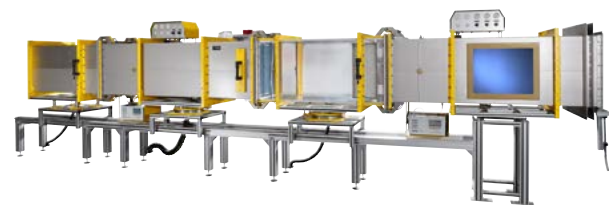
Filter test bench according to EN779:2012 / ISO 16890 / Ashrae 52.2
