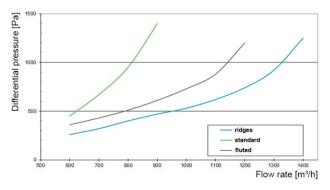
Comparison of differential pressure development on load with fluted filter media, with and without the pleat distance control with the Filtration Group technology of ridges
