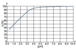
Filtration efficiency: > 98 % at 6  $\mu m$
