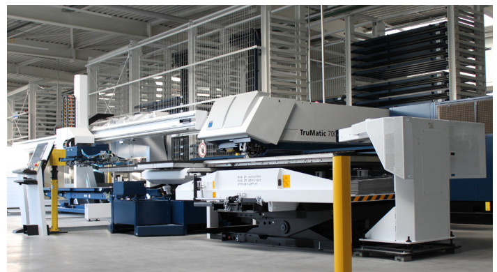
Punch-laser combination machine with storage system. Both machines require compressed air. Picture source: Pfister Metall
