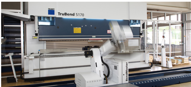
Edging robot with vacuum gripper. Numerous machines operate with compressed air.
